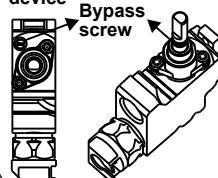
**Valve without flame failure device**
