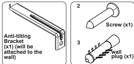
The document bag contains an anti-tilting kit. Loosely attach the anti-tilting bracket (1) to the wall using the screw (2) and wall plug (3), following the measurements shown in the figure and table below. Adjust the height of the anti-tilting bracket so that it lines up with the slot on the cooker and tighten the screw. Push the appliance towards the wall making sure that the anti-tilting bracket is inserted into the slot on the rear of the appliance.
