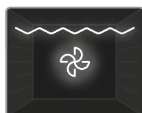
**Grill and Fan Function:** The oven's thermostat and warning lights will switch on, and the grill heating element and fan will start operating.
